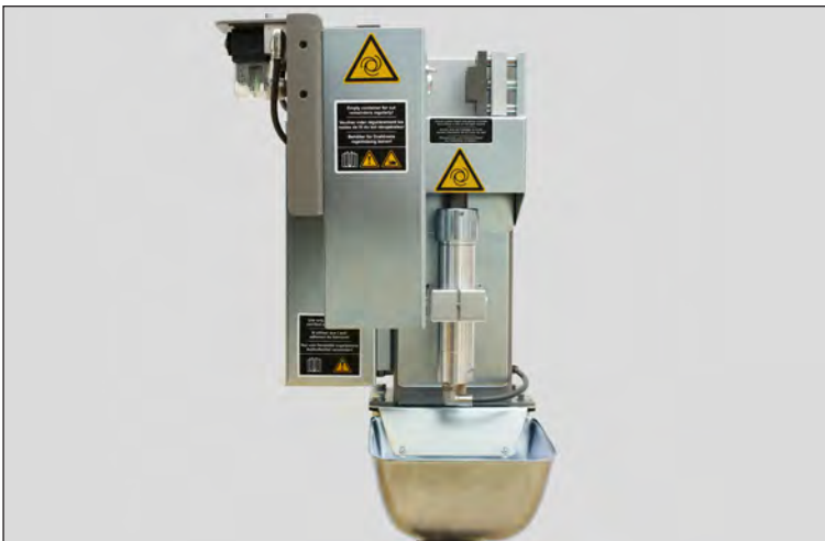
Optional with wire cutter DIX PRA 600 and assembly fixture DIX PRF 600
